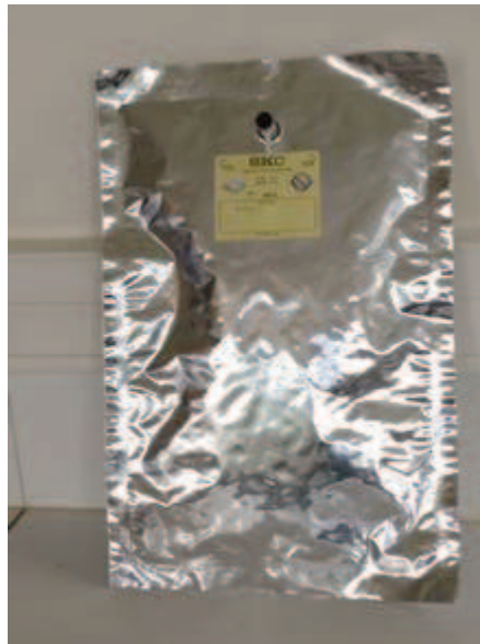
Figure M5.1. Flexfoil® sample bag used for sampling the air in livestock buildings (source INRA)
