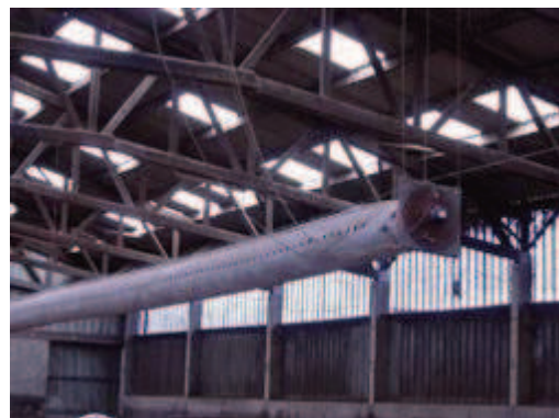
Figure M14.1. Duct for dispersing the tracer gas within a building (source: INRA)
