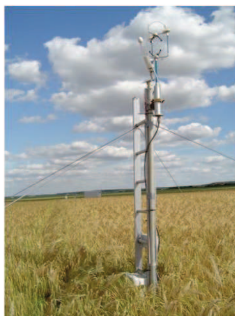
Figure M31.1. Eddy covariance system for measuring CO 2 fluxes (INRA)
