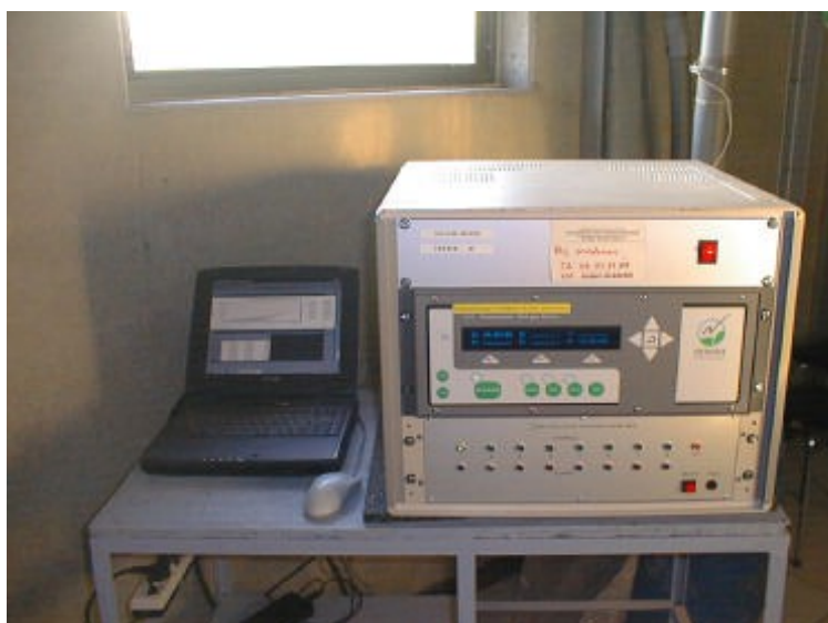
Figure 3. Photo-acoustic multi-gas monitor with 6 channel multi-sampler
